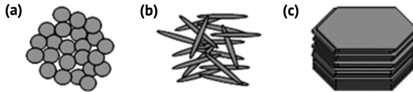
Figure 2.1: Types of nanofillers according to their geometries: (a) spherical, (b) rod-like, and (c) platelet-like nanofillers (adapted from reference [18]).
